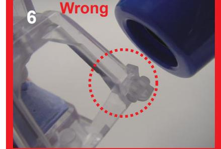
The bite adjustment heat gun facilitates easy re-articulation for cases in which the patients' bite is wrong. The bite can be adjusted in less than 1 minute by simply softening the neck of the hinge with the heat gun and then re-articulating. Heat the neck area (the yellow circled area) of either the opposing tray or the working tray for about 15 to 20 seconds. During this time, be sure to switch teeth every 5 to 6 seconds so that the neck area may be heated evenly. (Pic. 1 & 2)
