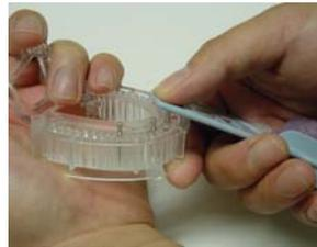
As seen in the hands-on video, the dowel pins may be pushed down into the pinholes by using a tool such as the back of an impression handle or simply by pushing the pins down with your thumbs. Make certain that you do not push the pins down into the pinholes with excessive force. When the ceramists re-insert the pinned dies onto the articulator throughout the fabrication
