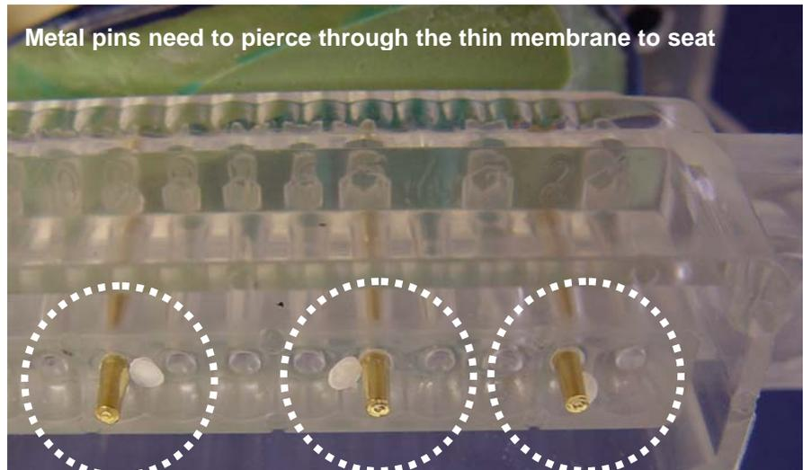
Metal pins need to pierce through the thin membrane to seat
