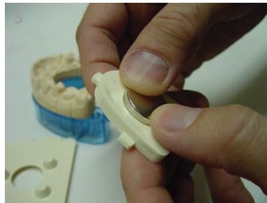
(Insert the magnet) Push the magnet all the way down into the hole on the magnet housing plate .
