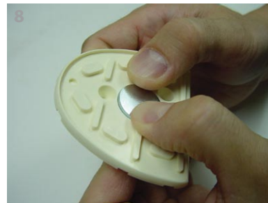
(Insert the metal piece) Push the metal piece into the metal housing plate from the bottom of the plate.
