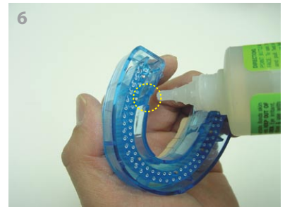
(Glue for the magnet housing) Place a drop of glue in each of the 3 slots located on the bottom of the working tray.
